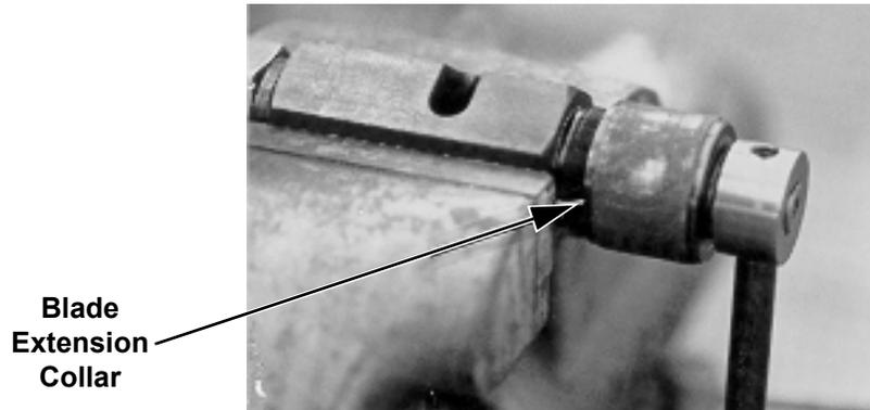
3. Clamp the coning tool in a vise.
