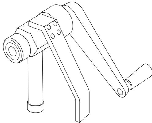
**Old style** The old style coning tool (part number 26160-xxx) requires different replacement collets and blades, and a separate tool is required for each tubing size. Replacement parts for older style coning and threading tools:
